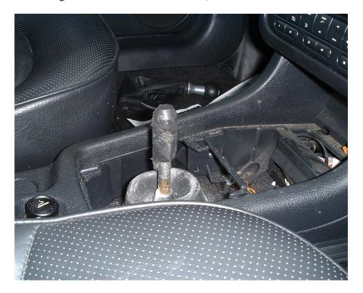
Then it's just a matter of whittling down the rubber until you can just about force the gear knod over it. You don't want it too slack or you'll have to glue the knob on to stop it swivelling and then it will be very hard to replace. Here's the rubber whittled down.
