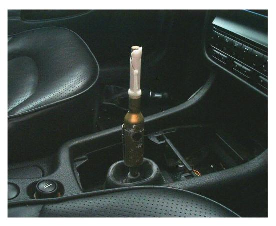
Then using a junior hacksaw again, I cut down the length of the brass coloured section of aluminium and using a stanley knife, separated it from the rubber underneath.
